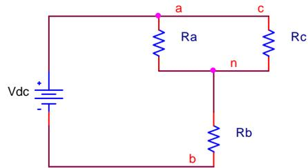
1. What is the line to neutral voltage across each phase of the load? i.e what's  $V_{an}$ ,  $V_{bn}$ , and  $V_{cn}$ ?
