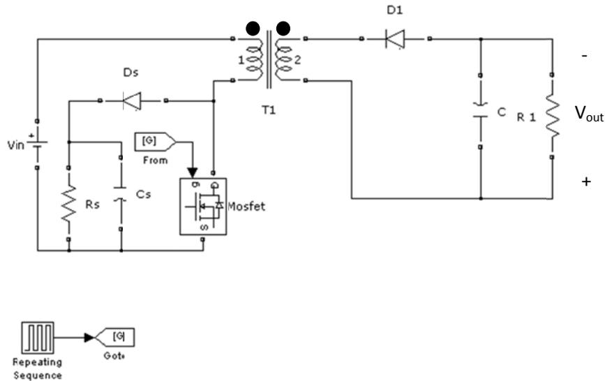
**Circuit 4** Flyback converter with RCD snubber
