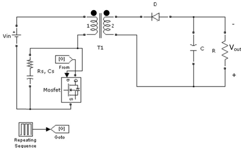
**Circuit 3** Flyback converter with RC snubber
