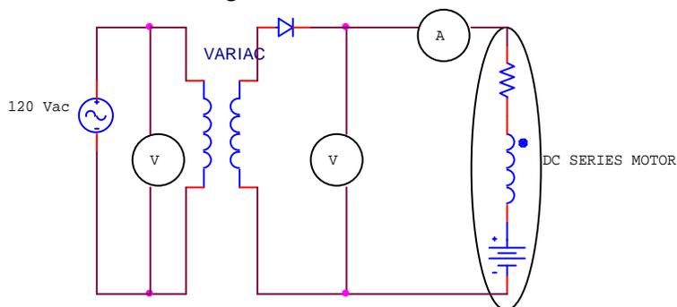
3. Set up the LVDAC-EMS scope to monitor both voltages and the current simultaneously.
